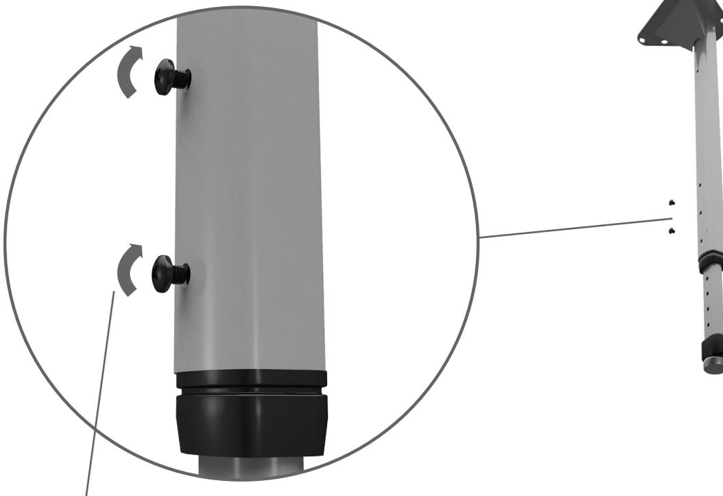
**DO NOT USE POWER DRILL TO APPLY** 10-32 x 3/16" **phillips** Screws. They will **STRIP OUT**
