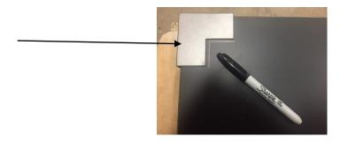
REMOVE FILM FROM DOUBLE FACED TAPE THAT IS APPLIED TO THE METAL FRAME. ALIGN FRAME WITH MARKS AND PRESS DOWN FIRMLY.
